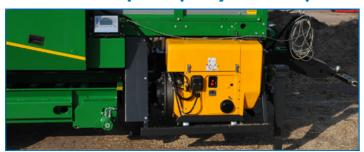
Cost effective operation through a direct connected diesel engine with low fuel consumption. Engine installed as a silent pack on the baler which makes use very simple as well mobile as stationary.
