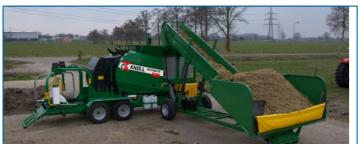
When loading capacity is a requirement. Loading volume is 2,5-3 ton. Conveyor width 1,20 mtr. Direct unloading from wagon into dropbunker.
