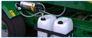
Fully automatic additive system voor adding additives during baling. Pump capacity 10 l/min.
